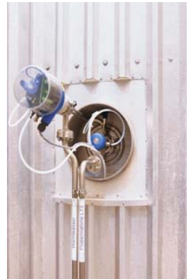
The valves are installed flush with the tank, which allows optimal cleaning on the tank side.
