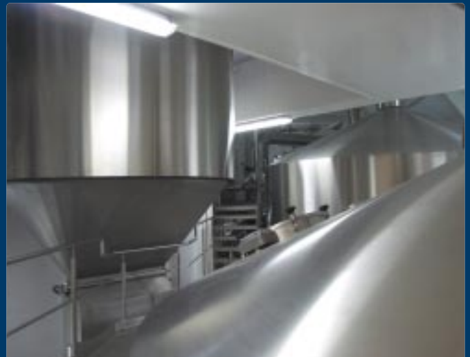
The hopper above the Millstar mill is on the left with the mash conversion vessel in the right foreground. The lauter tun is beside the steps.
