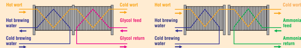
Fig. 12.3 – right: Two-stage wort cooling with direct ammonia cooling in the post-cooling stage
