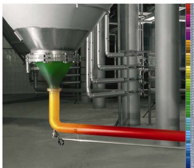
Figure 2. Temperature distribution in the outlet pipe.
