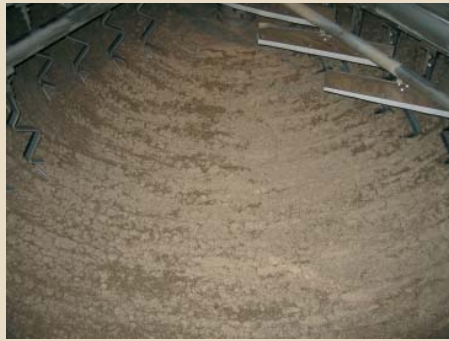
Fig. 1b Even spent grains bed with mashing off from below
